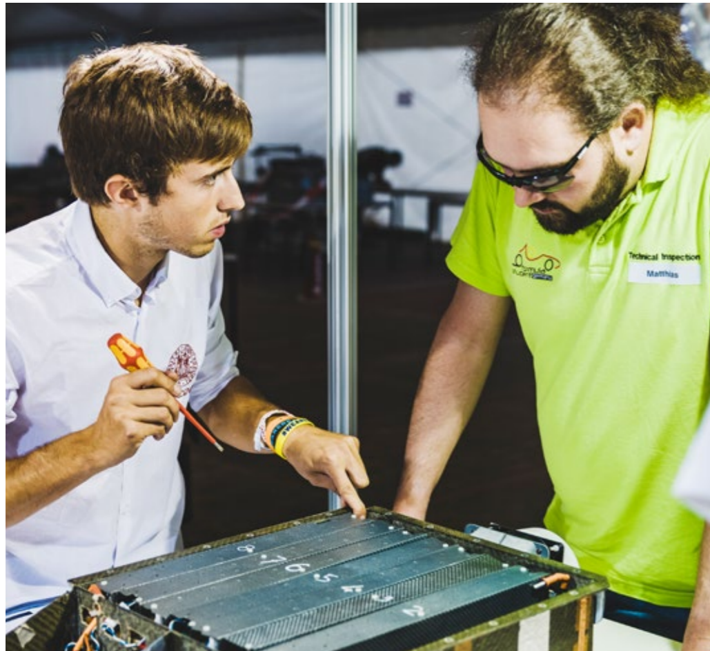
During E-Scrutineering the accumulator is checked extensively.
