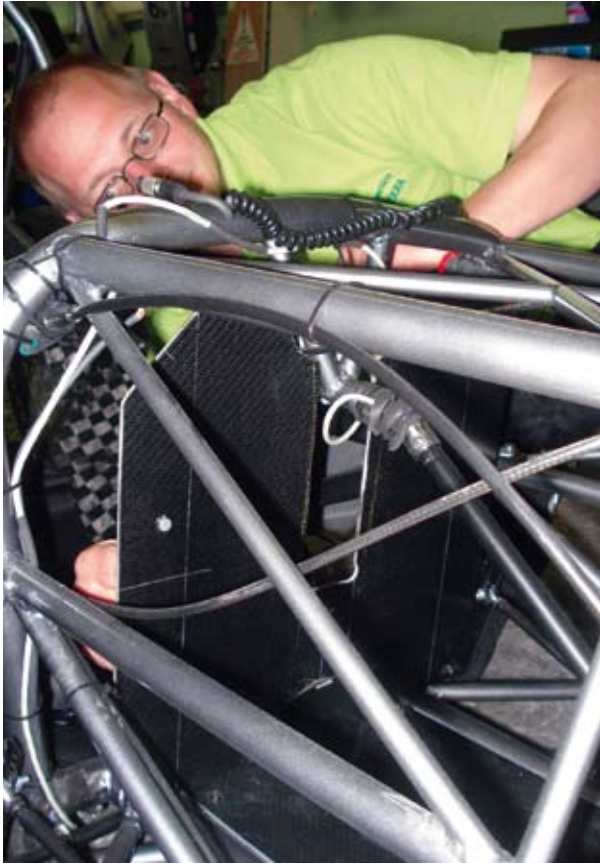
above: The foot well template needs to pass down to the driver's foot position. right: The measures of 'Percy', cockpit opening and foot well template are established in the rules.
