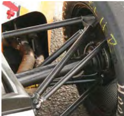
Carbon composite suspension members and road wheel on TU München car 2007
